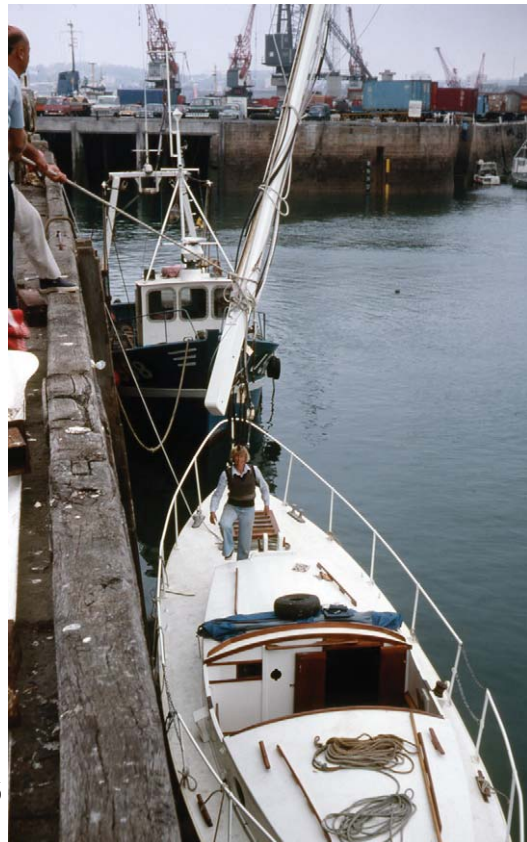
Re-stepping the wooden mast after it had been opened and re-glued
